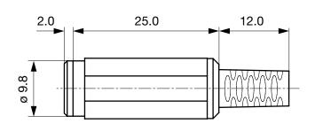
Cable diameter max. 4.0 mm
